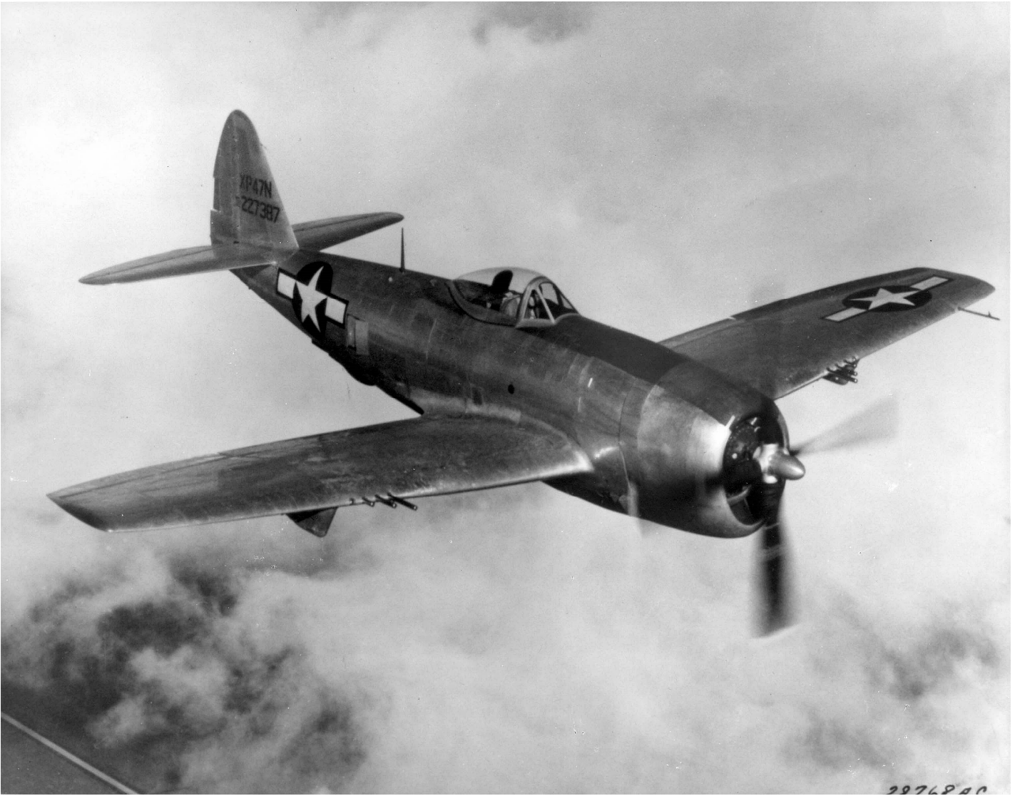
The P-47N, the last Thunderbolt variant to be produced. It was designed as an escort fighter for the B-29 Superfortresses being used in bombing raids against Japan.
