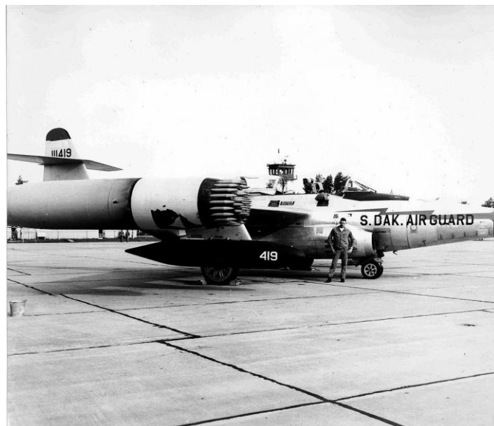
F-89D loaded with rockets, 114 th Fighter Interceptor Group, 1958 Photo credit: John Mollison, South Dakota Air National Guard
