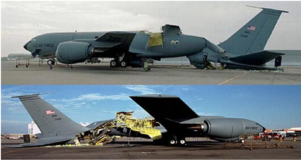
Two views of the stricken KC-135 Stratotanker after faulty pressure test. Photo credit: U.S. Air Force
